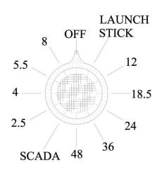
The 2-1/2 hour setting will empty the Launcher in 24 hours. The 5-1/2 hour setting will empty the Launcher in 48 hours. The 18-1/2 hour setting will empty the Launcher in one week.
